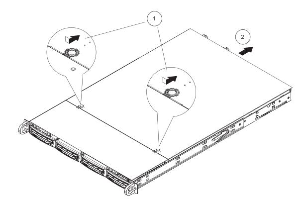
Figure 2-5. Accessing the Inside of the System
